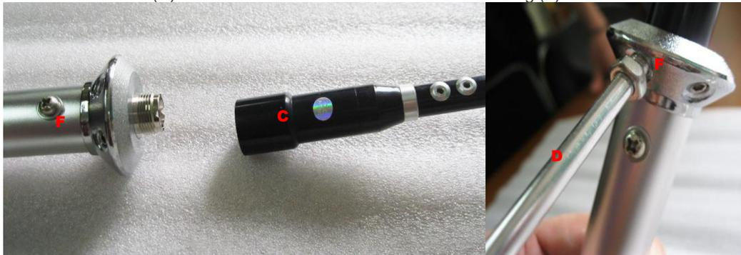
8. Mount Assembled Antenna to Cable Housing (F) to Mast using U-Bolts and Mounting Plate (G)
